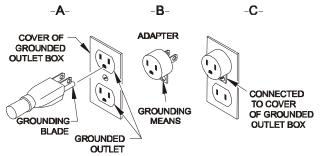
NOTE: The use of the adapter shown in Figure B and C is not permitted in Canada. If a grounding type receptacle is not available, do not use this charger until the proper outlet is installed by a qualified electrician.
